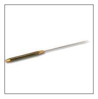
The bodkin can serve two purposes. The first is to pick out material to give a more buggy appearance. The second is the application of head cement. You can create your own. A long needle or a bamboo skewer works fine.
