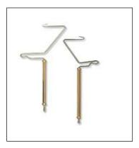
The whip finisher is designed to finish off the fly. It can be replaced with the dextrous use of hand tied half hitches.
