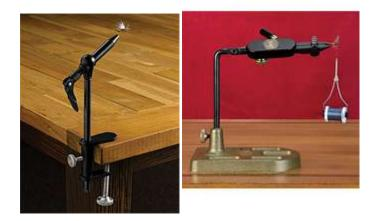
The vise on the left sells for about \$39.00 and has a fixed head. The one on the right sells for about \$200.00 and has a rotatable head.
