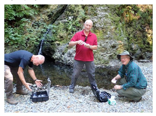
In the picture are three of the club's "A" team with Ton on the YSI meter, which measures temperature, dissolved oxygen and conductivity, while Ant is filling the sample bottle for Dan to use in the turbidity meter.
